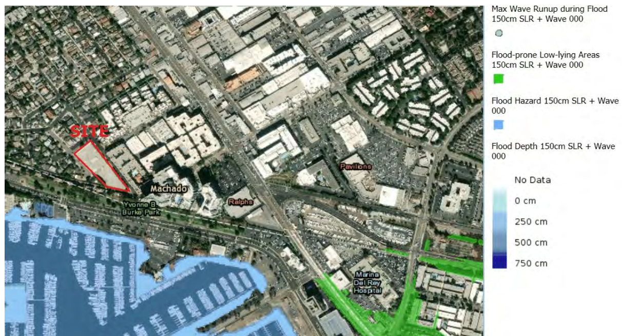
Figure 4. CoSMoS output for 4.9 feet of SLR at the site in the Venice Area.
